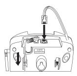
5. Place the cord inside the molded channel on the bottom of the Base Unit.
